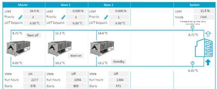
Plant overview, with real-time data Full insight in the plant operation for commissioning and optimization.
