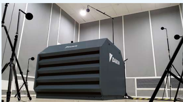
Sound power level measurement in acoustic chamber
